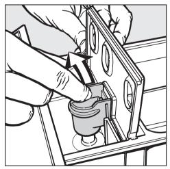
■ Remove the siphon tube from compartment <sup>1</sup>/<sub>2</sub>.
